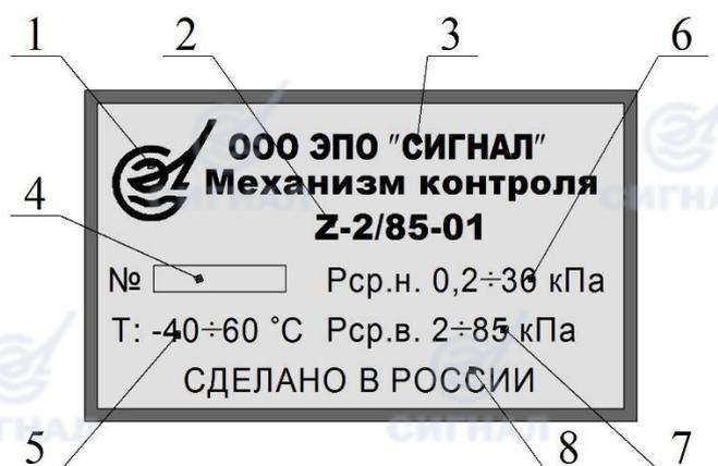
The image shows a rectangular label for a control mechanism. It contains the following information: a logo (1), the manufacturer's name 'ООО ЭПО "СИГНАЛ"' (2), the mechanism model 'Механизм контроля Z-2/85-01' (3), the factory number '№ [ ]' (4), working temperature range 'Т: -40÷60 °С' (5), adjustment range for decrease 'Рср.н. 0,2÷30 кПа' (6), adjustment range for increase 'Рср.в. 2÷85 кПа' (7), and country of origin 'СДЕЛАНО В РОССИИ' (8).
